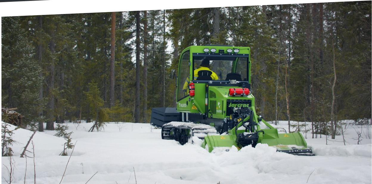
Thanks to the minimal ground pressure, low centre of gravity and high ground clearance, the machines are capable of operating in difficult conditions, such as snow and crossing deep ditches.
